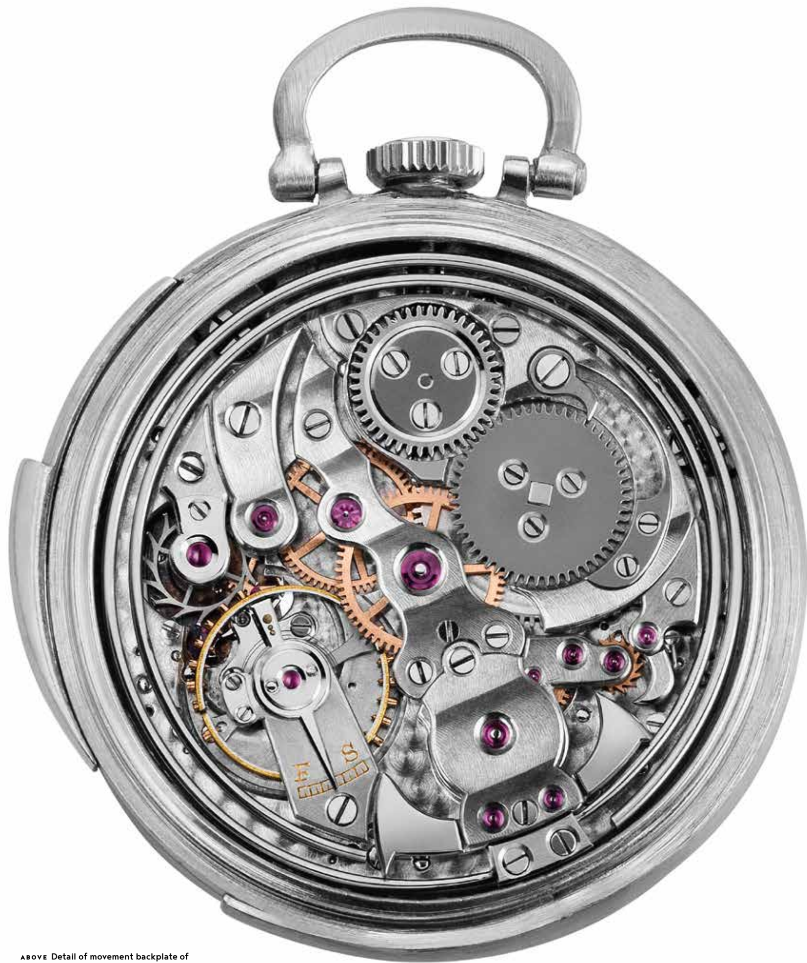
Above Detail of movement backplate of an Audemars Piguet, made in 1912. A platinum open-faced keyless lever watch with minute repetition (cal. 9½ SMV #61) Diameter 25 mm
