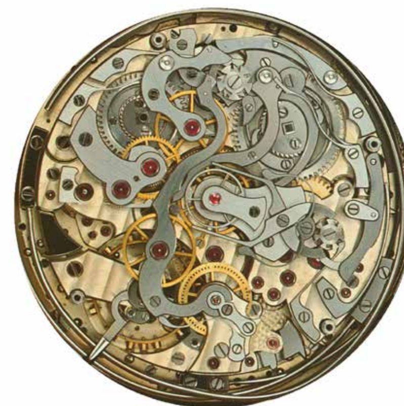
TIER 1 - UNDER SIDEREAL TIME DIAL VIEW WITH SIDEREAL TIME TRAIN REMOVED SHOWING THE TIME AND CHRONOGRAPH MECHANISMS
